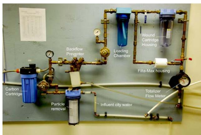
**Figure 1.** Apparatus for spiking filters in the laboratory.
